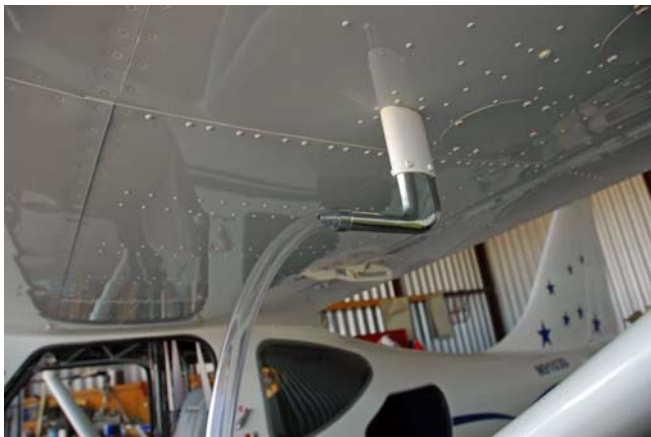
Dennis' Pitot after Manometer Calibration
